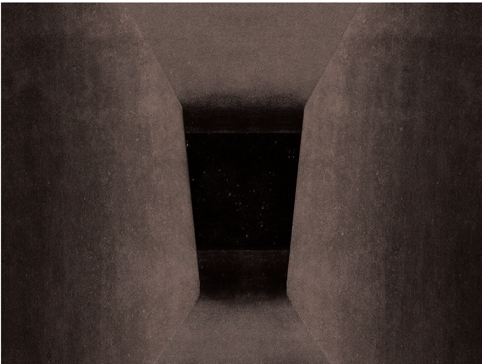
Figure 6: Corridors library – Category V2 'Variation of section layout': Study sketch of the case 2.4 (trapezoidal section with externally-inclined walls)
